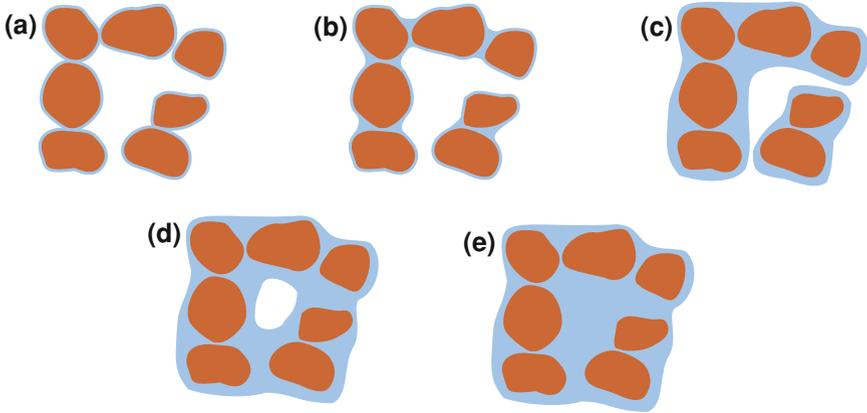
**Fig. 2.2** Spatial configurations of water and air in an unsaturated granular porous medium: **a** adsorbed regime, **b** capillary pendular regime, **c** capillary funicular regime, **d** occluded air bubble regime, **e** fully saturated regime
