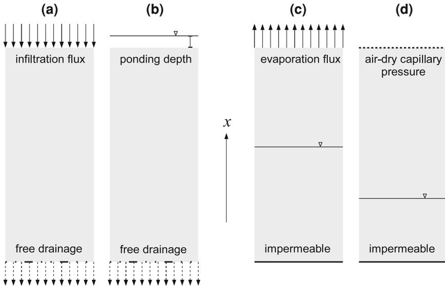
**Fig. 2.9** Boundary conditions for typical one-dimensional flow problems: infiltration towards a distant groundwater table, **a** early stage, **b** late stage; evaporation from shallow groundwater table, **c** early stage, **d** late stage
