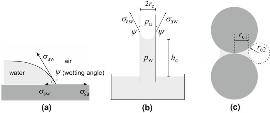
**Fig. 2.1** Surface tension effects: **a** equilibrium position of the fluid–fluid interface near the solid surface, **b** rise of the wetting fluid in a capillary tube, **c** pendular ring around the contact point of two solid grains
