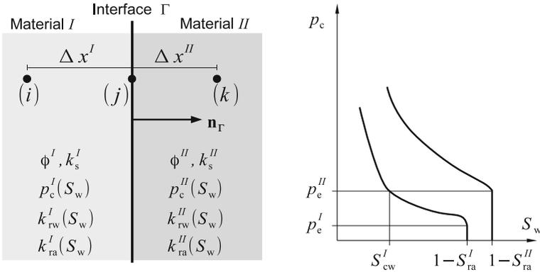
**Fig. 2.10** Conditions at material interface separating two porous media
