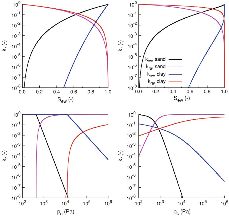
**Fig. 2.6** Typical relative permeability functions for sand and clay according to Brooks–Corey–Burdine model (*left*) and van Genuchten–Mualem model (*right*). At the *top*  $k_r(S_{ew})$  functions, at the *bottom*  $k_r(p_c)$  functions
