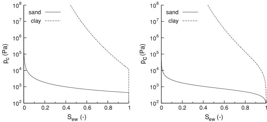
**Fig. 2.5** Typical capillary functions for sand and clay
